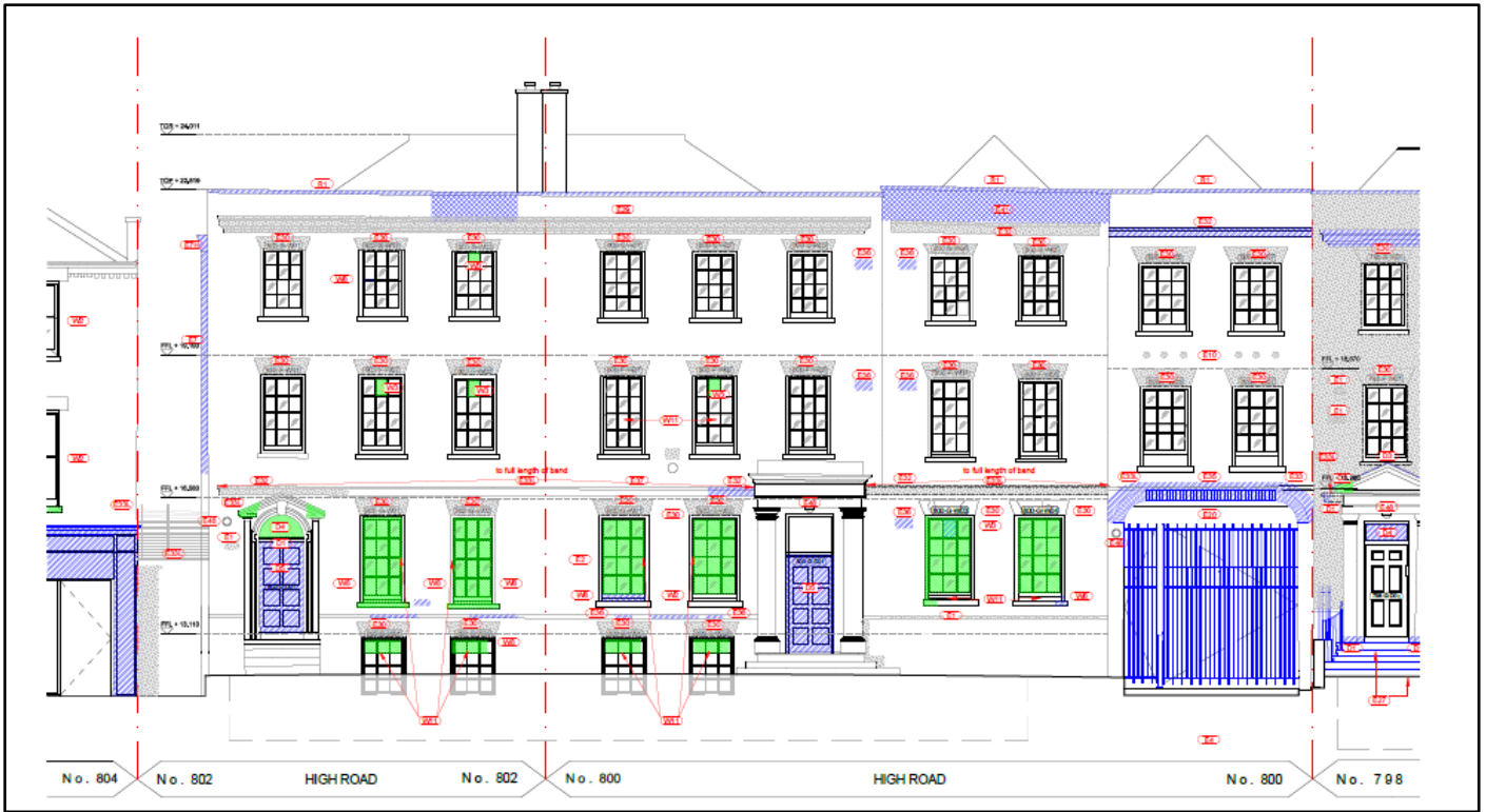
Conservation repairs to all High Road elevations (Nos. 800-802 shown here)
