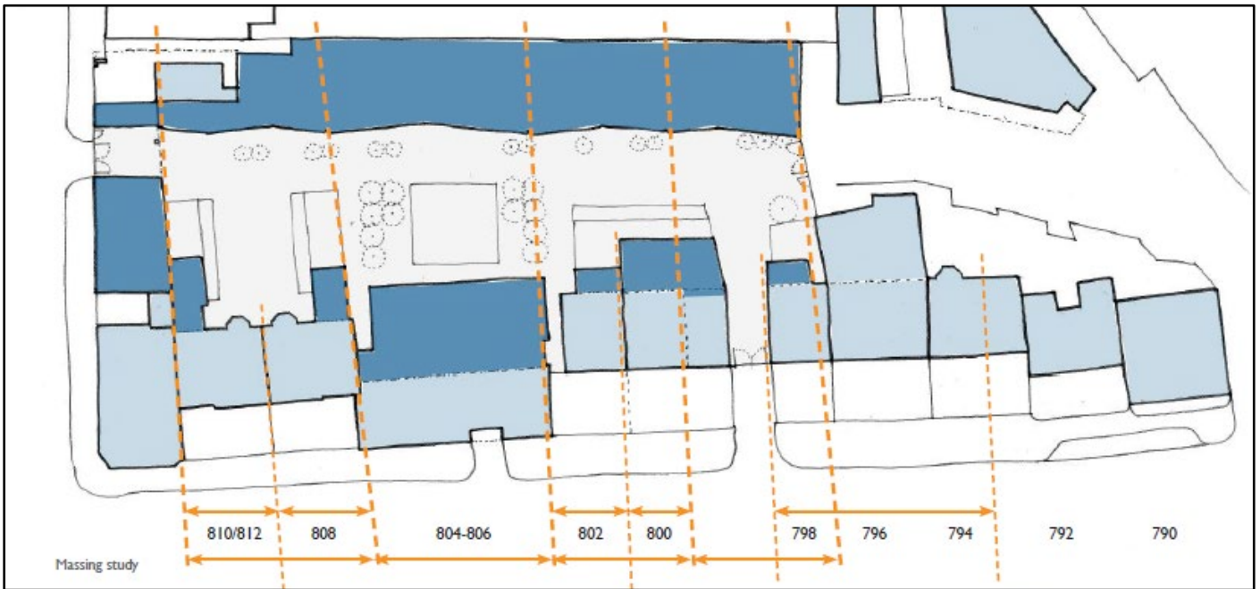
Sketch plan showing proposed 'Linear Building' and refurbished and extended High Road buildings
